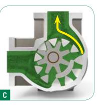
The R internal gear pumps are self-priming positive displacement rotary pumps perfect for viscous liquids (0,5 to over  $500.000 \, \text{mm}^2/\text{s}$ ) of any temperature ( $-60^{\circ}\text{C}$  to  $350^{\circ}\text{C}$ ), which can be corrosive, abrasive and dangerous for the environment. The pumps are used for transferring, dosing, processing, loading and unloading.
