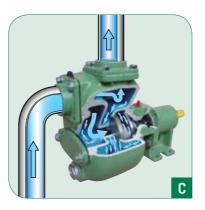
The S series pumps are centrifugal and self-priming. The impeller with open blades allows a wide passage of solids. With this kind of pump you can handle wastewater also with corrosive and viscous liquids containing solids in suspension, abrasive powders, even if there are air bubbles.
